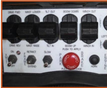
■ All cab controls can be found on the well-laid out wireless remote control console.
